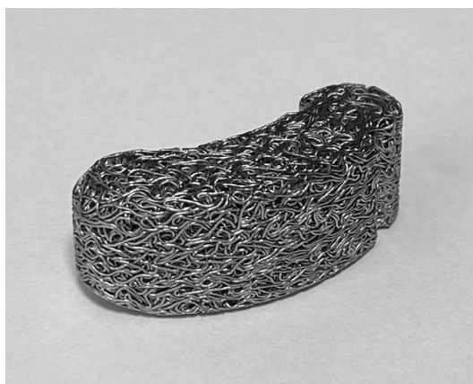
Figure 1. TFMB® Titanium cage (KYOCERA Inc., Japan). It is made by compression molding and vacuum sintering of pure titanium wire.
